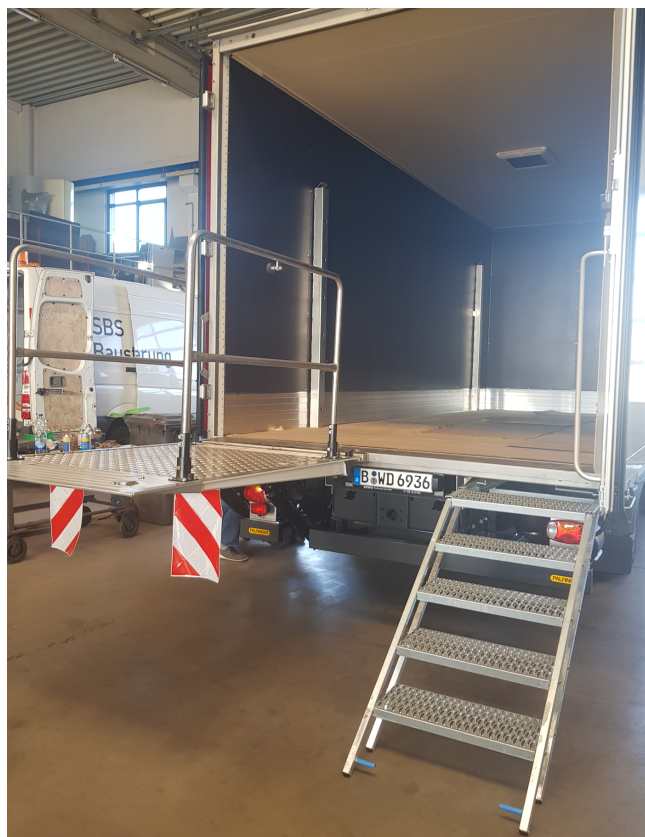
Figure 3: Access to the trailer with stairs and a secured loading ramp for wheelchairs.
