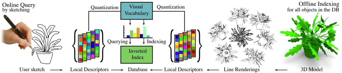
**Figure 3: Overview of our 3D shape search engine.** The offline shape indexing and online querying stages differ only in the way we generate input feature lines: automatic line rendering from 3D shapes (right) or hand-sketched by users (left).
