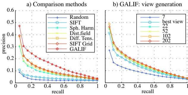
**Figure 9:** Detailed evaluation of retrieval performance on test dataset (higher curves are better): a) comparison with previous work using optimized system parameters; b) GALIF descriptor: influence of view generation methods.
