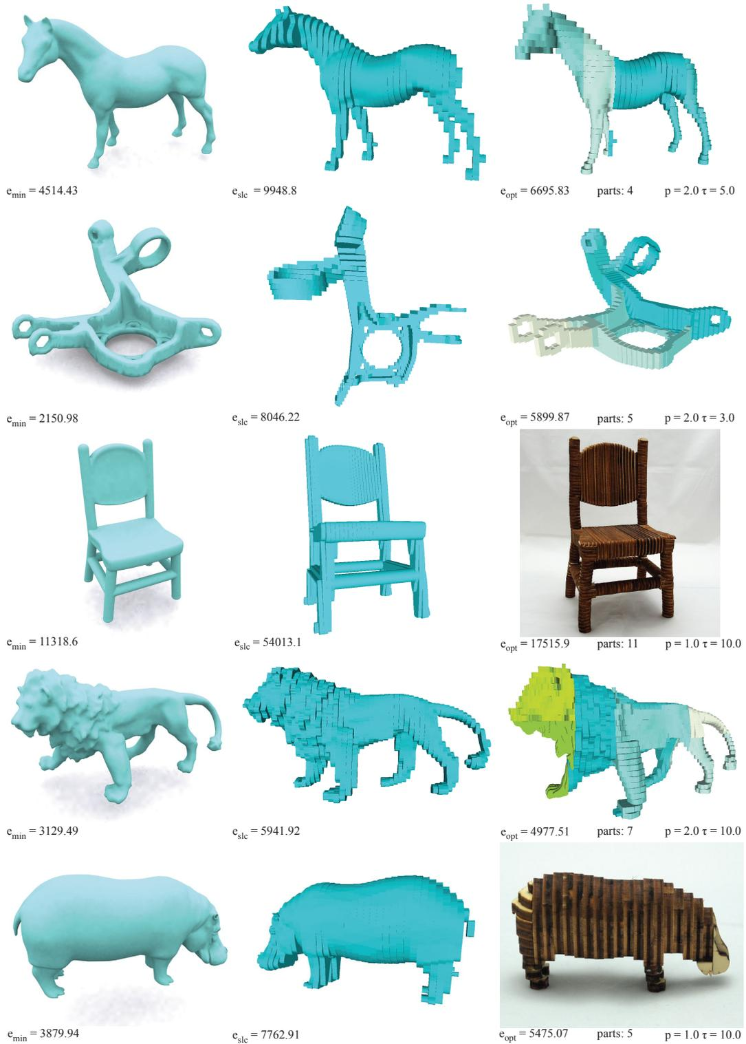
Figure 9: We show the input 3D shapes (left), a result that is sliced in its best direction (middle) and the handcrafted or 3D printed results or rendered images (right). We also show the best approximation error, the error that would result from one directional slicing and the error after optimization. Additionally parameter settings and the number of resulting subparts are annotated.
